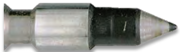
WITHOUT Fuel Maximizer Plunger Rating - Untreated Average 23.38%
